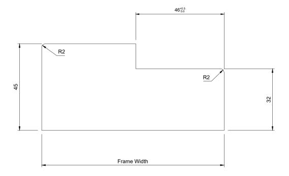
Do Not Scale. Description: Purchasing Profile Timber System 2 - 45/32 Profile - NFR - 44mm Door - Non-Acoustic - Non Q2F
